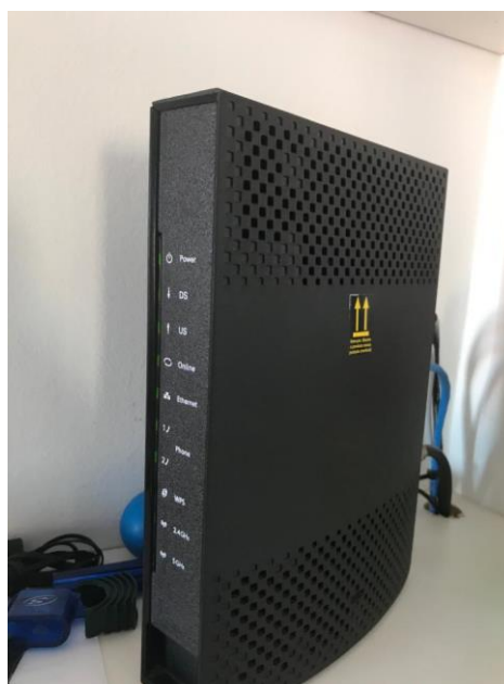
Figura 2 – Cable Modem Technicolor 7337.
